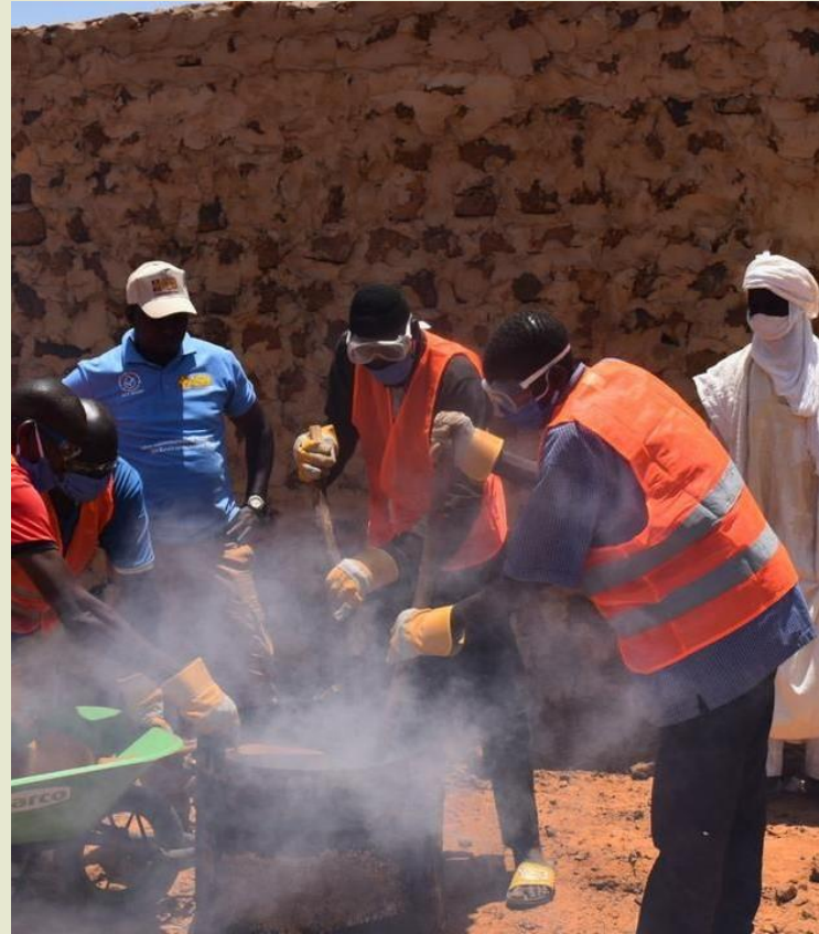
2 · Melt it in metal drums, with protective gear
